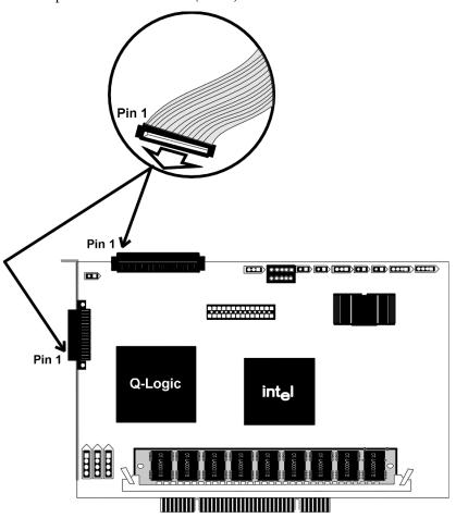
Connect SCSI Devices When connecting SCSI devices:
